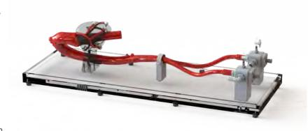
integrated hemostatic valves at the femoral arteries to facilitate insertion, advancement and delivery of coronary intervention implants. Additional custom access approaches through the radial artery can be further integrated into the simulation systems, along with calcified coronary arteries.
