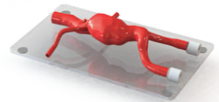
Sheet-base with hemostatic valves
