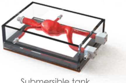
Submersible tank with hemostatic valves
