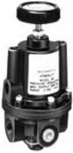
The Low Pressure Regulator is a precision pressure regulator designed for applications that require high resolution such as the RDTL-0200 System. The Regulator features control sensitivity of 1/8" water column, a pressure range of 0-10 psi, and a balanced supply valve to deliver consistent and reliable accuracy to maintain the system desired set point regardless of supply pressure changes or flow conditions.
